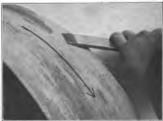
Fig. 267. Grinding a Skew Chisel.
